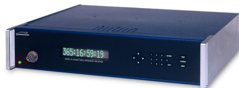
XLi SAASM GB-GRAM Time and Frequency Receivers (left: 1U model, right: 2U model)
